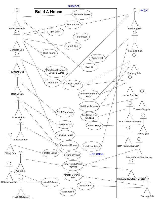
Figure 5-8: Use Case Diagram for the Operation of the Homebuilding Process
