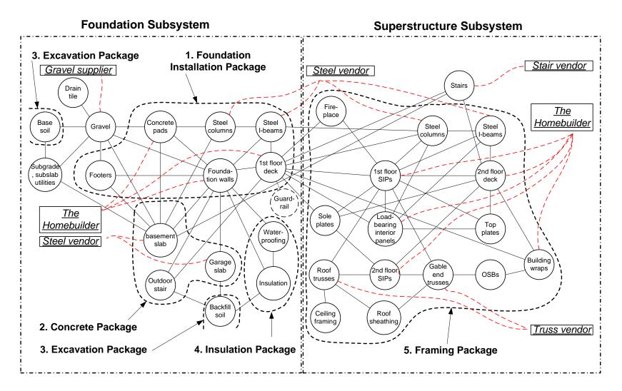
Figure 5-12: Overall Structure of Foundation and Superstructure Subsystems
