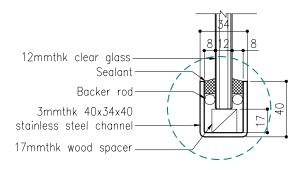
Figure 5-4: Glass Panel Bottom Sectional Detail
