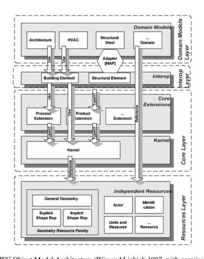
**Figure 2-8:** IFC Object Model Architecture (Wix and Liebich 1997, with permission from CIB) The IAI (1999a) has set up important representatives of information for the development of the IFC, such as classes, objects, attributes (information about the class or its interface), relationships (occurring between classes), interfaces, the object model, process diagrams, usage scenarios, and
