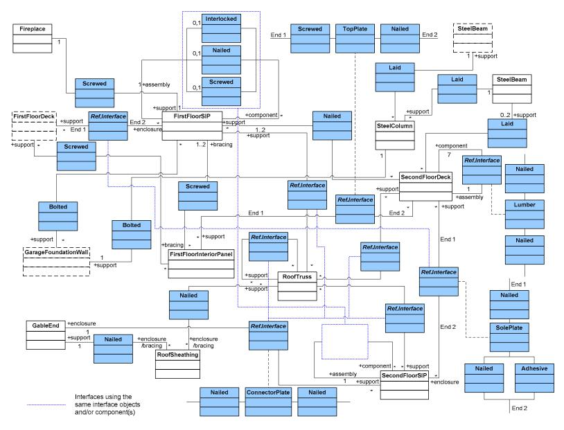
Figure 5-16: Interface Model for Componentized Superstructure Framing
