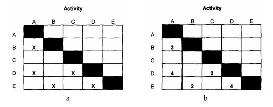
**Figure 2-6:** a) Partitioned Design Structure Matrix; b) Modified Information Matrix (Bogus et al. 2002, with permission from ASCE)
