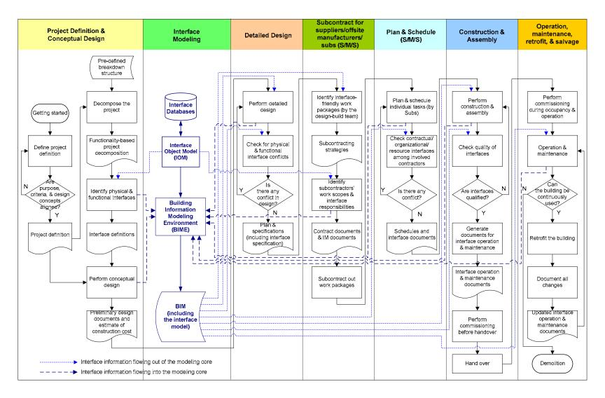
Figure 6-4: Systematic Model-Based IM Process Flow Chart
