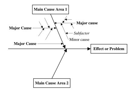
Figure 3-1: The Method of the Cause and Effect Diagram
