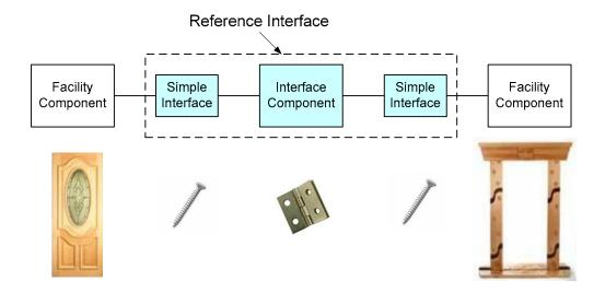
Figure 4-11: The Simple Type of Reference Interface
