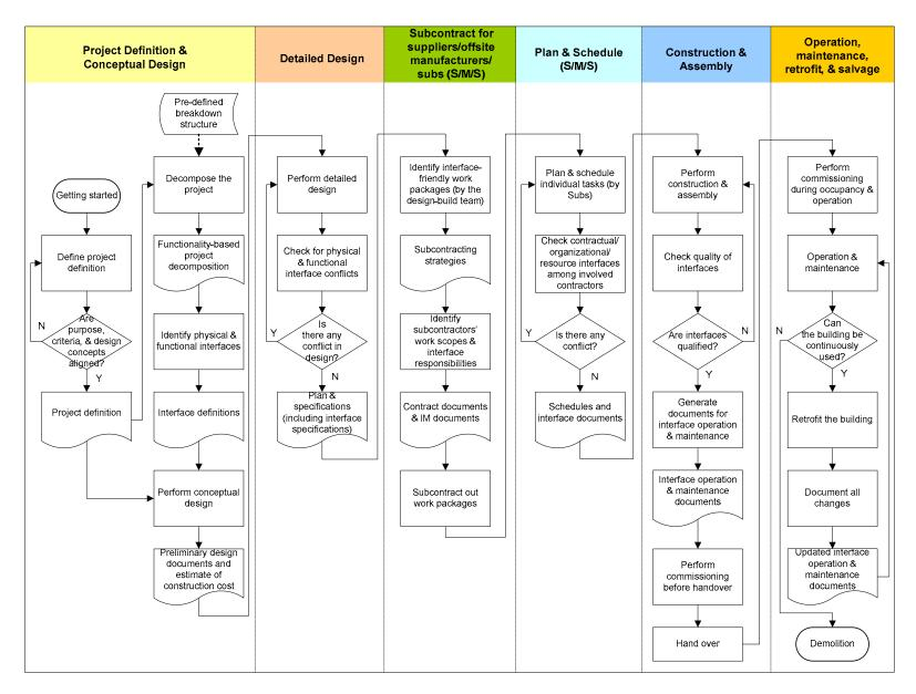
Figure 6-2: IM Sub-processes in a Complete Project Process
