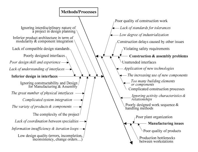
Figure 3-8: Interface Issue Cause Factors from the Methods/Processes Perspective
