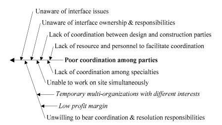
Figure 3-5: The Minor Causes for Poor Coordination
