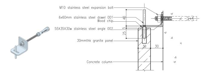
Figure 5-6: Granite Cladding Detail
