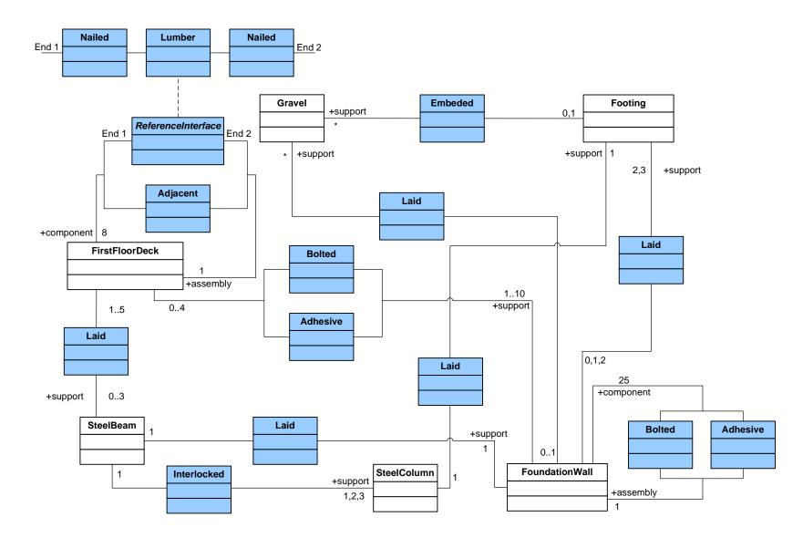
Figure 5-14: Interface Object Model for Foundation Wall Installation
