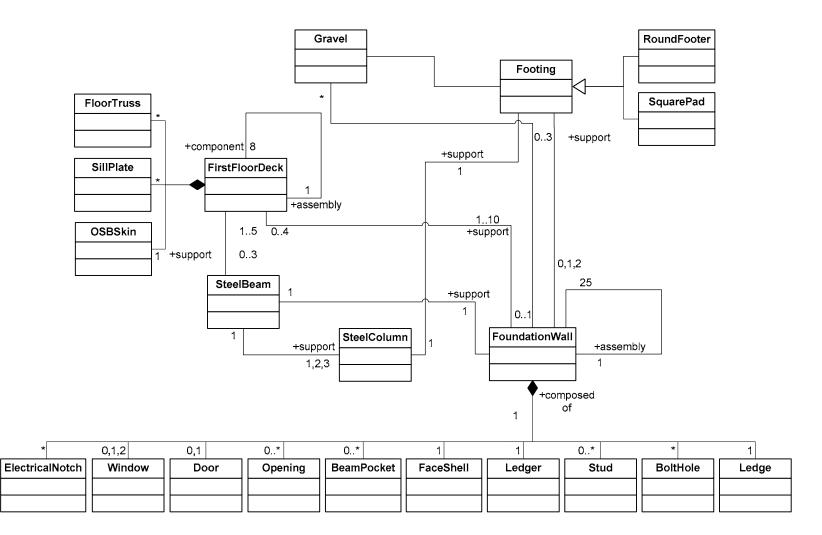
Figure 5-13: Facility Components and Their Relationships in Foundation Wall Installation
