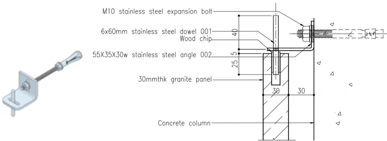
**Figure 5-6: Granite Cladding Detail**
