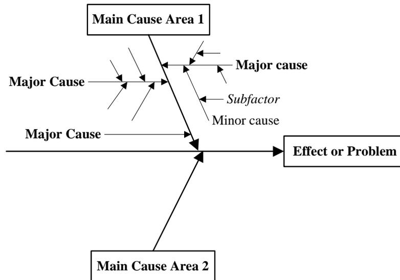
**Figure 3-1:** The Method of the Cause and Effect Diagram
