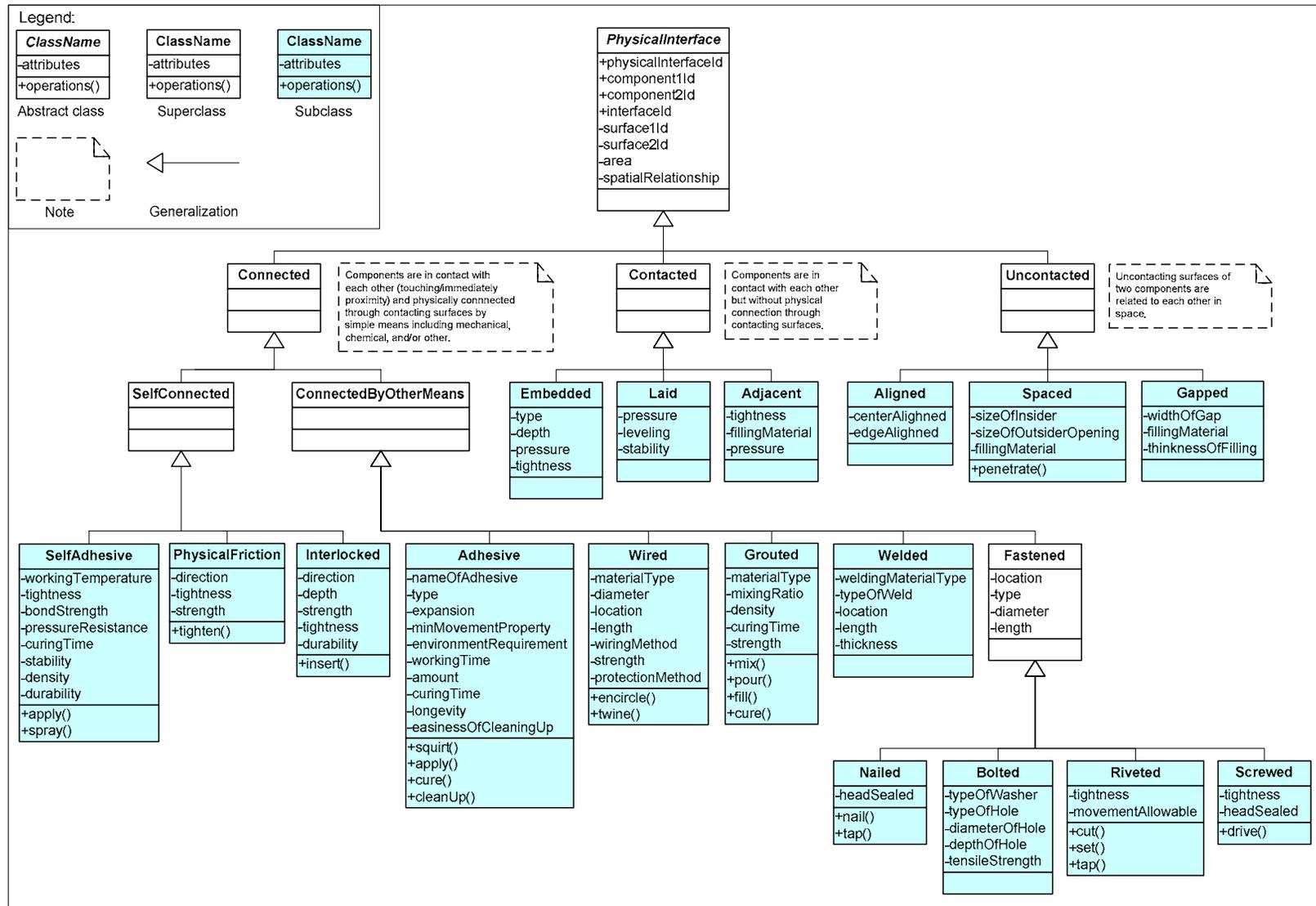
**Figure 4-6:** UML Physical Interface Object Class Diagram
