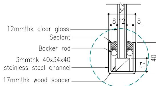
**Figure 5-4:** Glass Panel Bottom Sectional Detail
