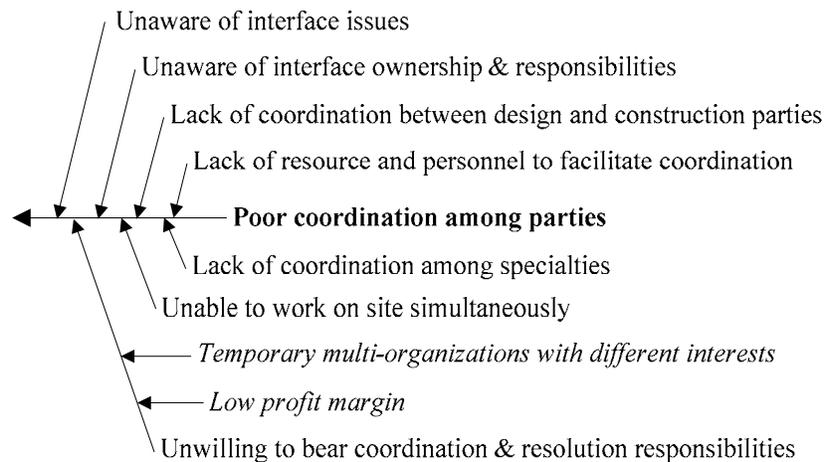
**Figure 3-5:** The Minor Causes for Poor Coordination
