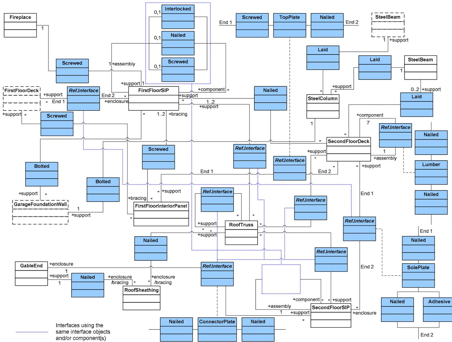
Figure 5-16: Interface Model for Componentized Superstructure Framing
