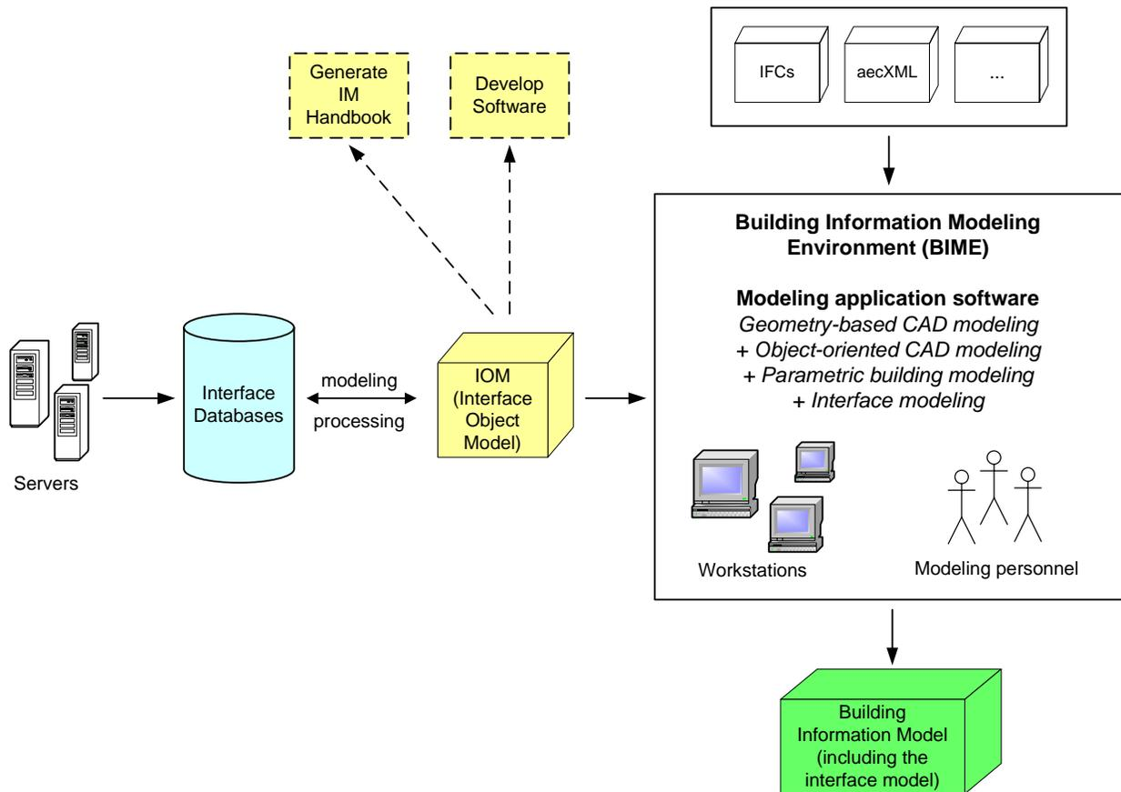
**Figure 6-3:** The Interface Modeling Core
