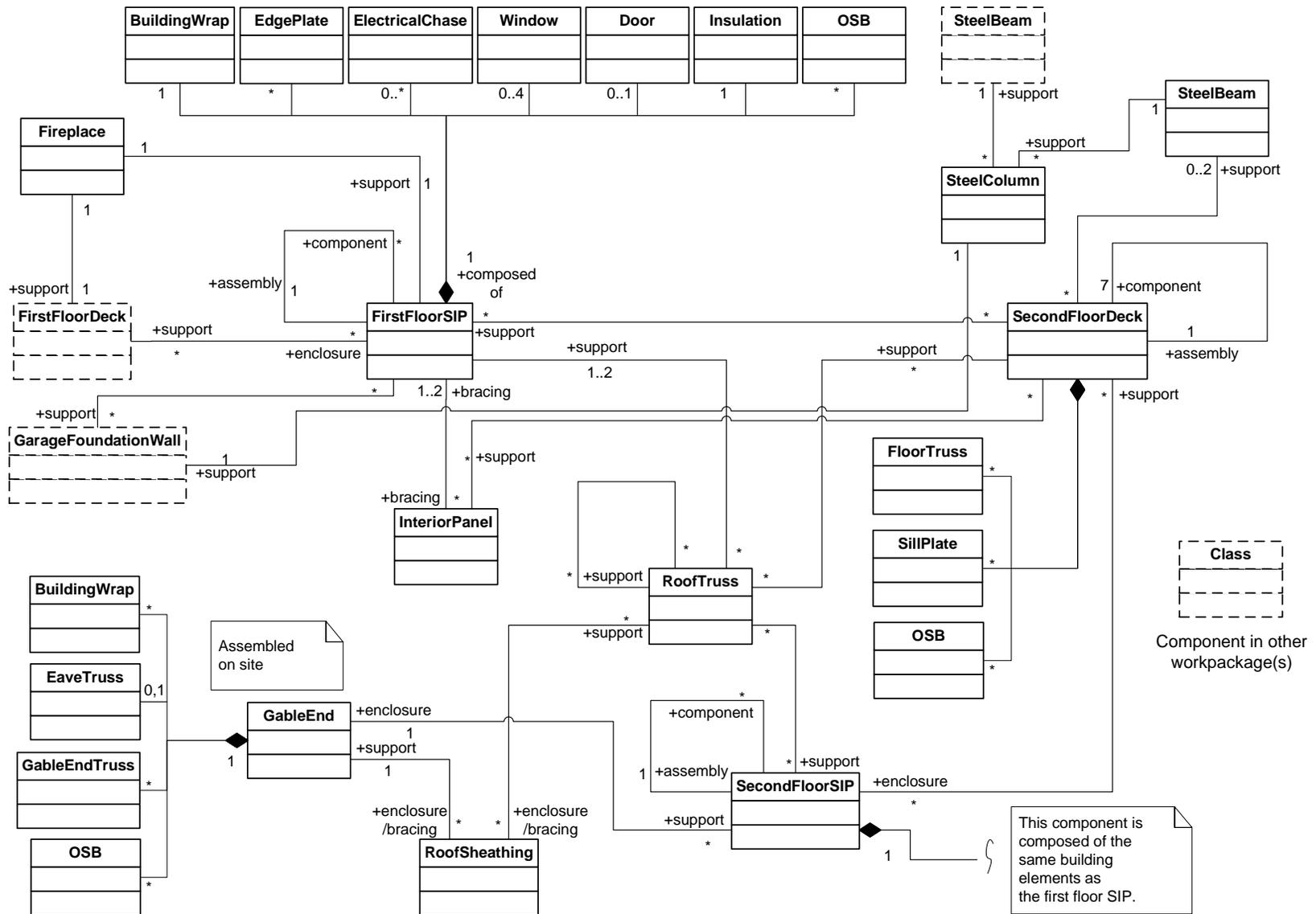
Figure 5-15: Facility Components and Their Relationships in Componentized Superstructure Framing
