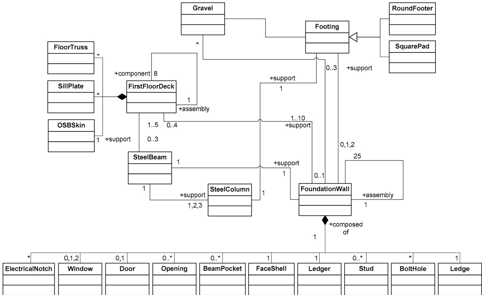
**Figure 5-13:** Facility Components and Their Relationships in Foundation Wall Installation
